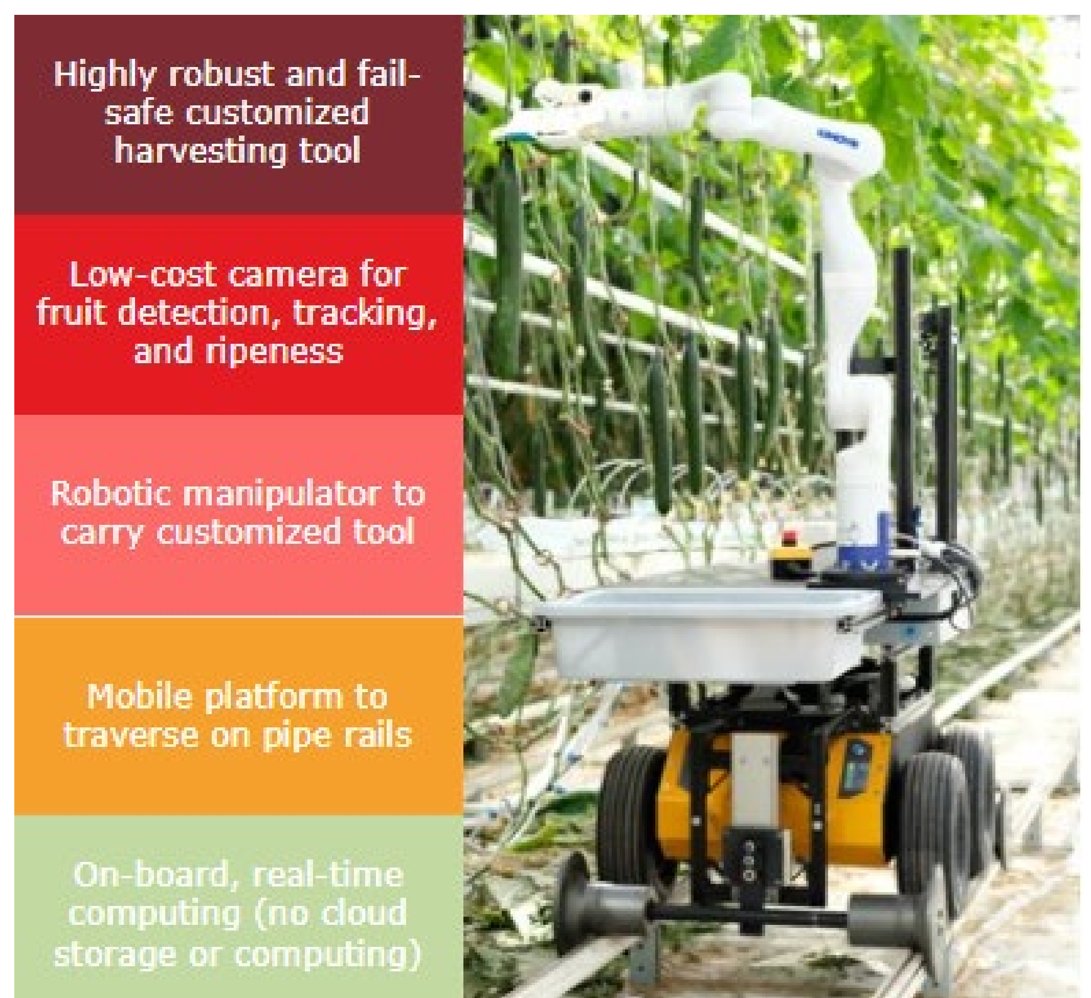
Figure 1 - Proof-of-concept vegetable harvesting robot and value proposition.
