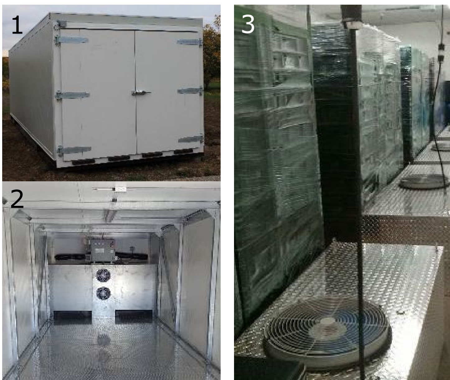
Figure 1 - Images 1 & 2 exterior and interior view of an enclosed chamber Appassimento unit. Image 3 free-air system.
