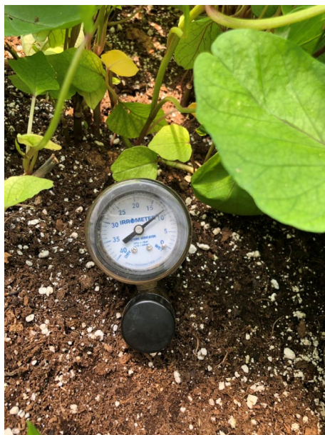
Picture 9: Tensiometer inserted in the soil to the depth of a sweet potato root seed.
