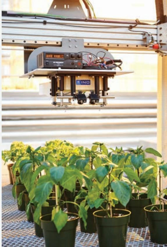
A smart irrigation system for potted plants is in development that will learn from a grower over a production cycle. PHOTO: VINELAND RESEARCH AND INNOVATION
